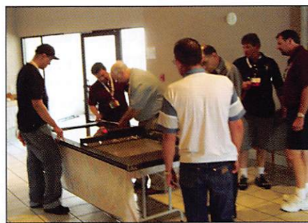
A student crew cuts the face off the door to accommodate the hardware.
