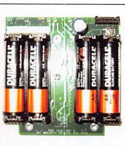
Photos show the electronic boards. The locks use 4 AA batteries.
