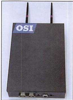
a pair of different portal gateways. These are the radios that communicate with the locks.
